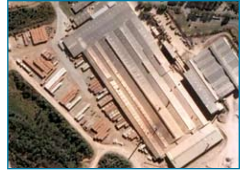
Aerial view of Austral Bricks' Rochedale Plant showing the 2ha of roof area to be used for stormwater harvesting
